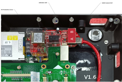
Typical installation of an indoor node
